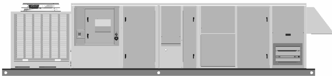
Extended Heat Recovery Cabinet
