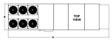
**Note:** Dimensions will be dependent on option content, and other field added features. Consult final selection drawings for complete details. Cabinets are available in vertical or horizontal discharge.
